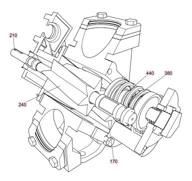
2. Remove the Pump Valve Housing and inspect the rotors for cracks and fouling. Replace as appropriate using Maintenance Procedure JC0346.
